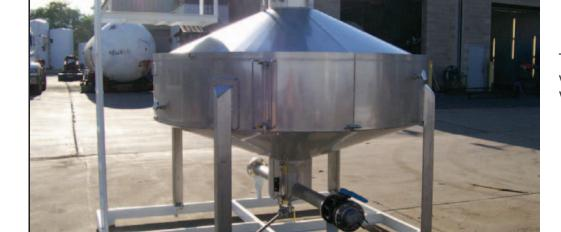
Tank Provers of varying sizes for 4" Volumetric Meters
